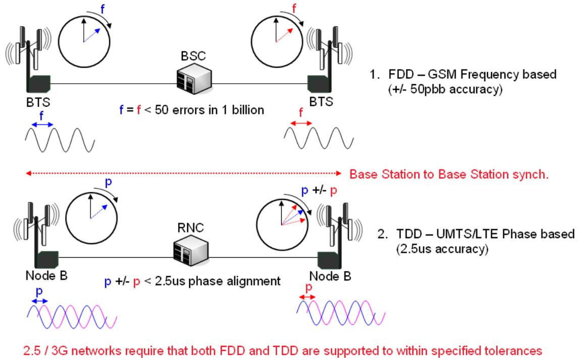
**Figure-5: Frequency and Phase Alignment**
