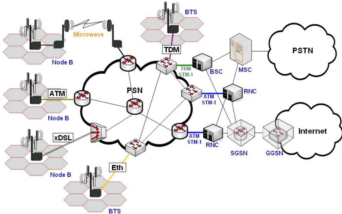
**Figure-4: GSM/UMTS Mobile Backhaul PSN**
