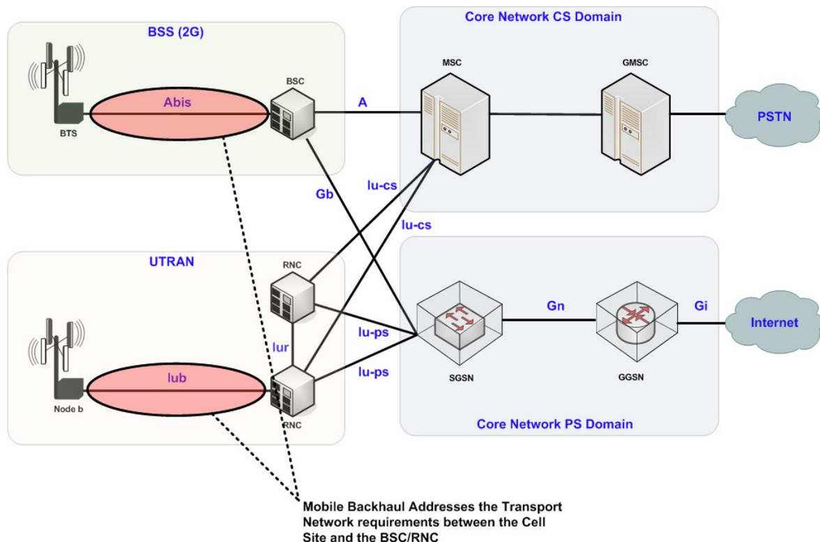
Figure-2: R99 GSM/UMTS Network Architecture
